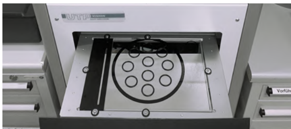
Dimensional, non-contact inspection using optical measuring machines
