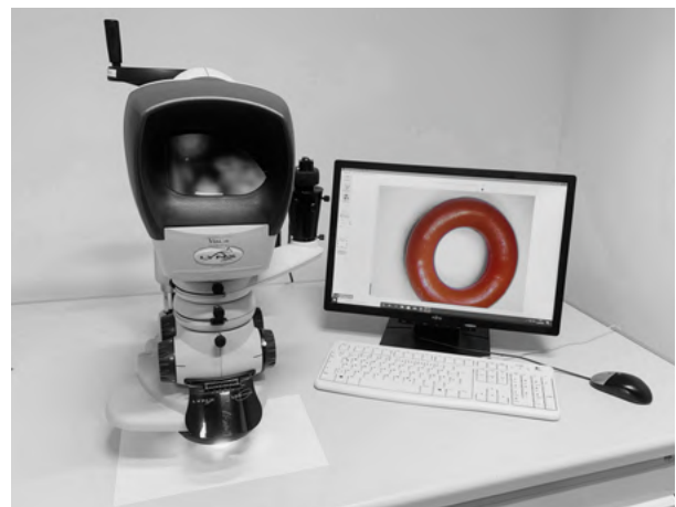
Surface inspection with a digital microscope
